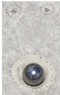
Figure 5: Passed dent from 3 in. diameter steel ball test compared to dents from a 1 ¾ in. diameter steel ball hail tests
