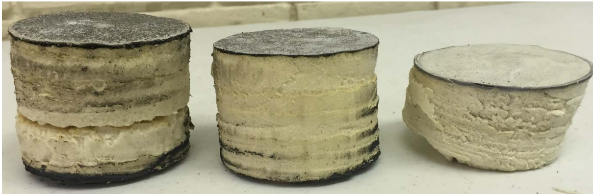
Figure 6: Passing, failing and new core samples
