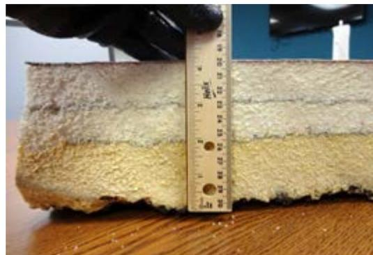
*Figure 2: Three Layers of SPF (4” thickness).*
