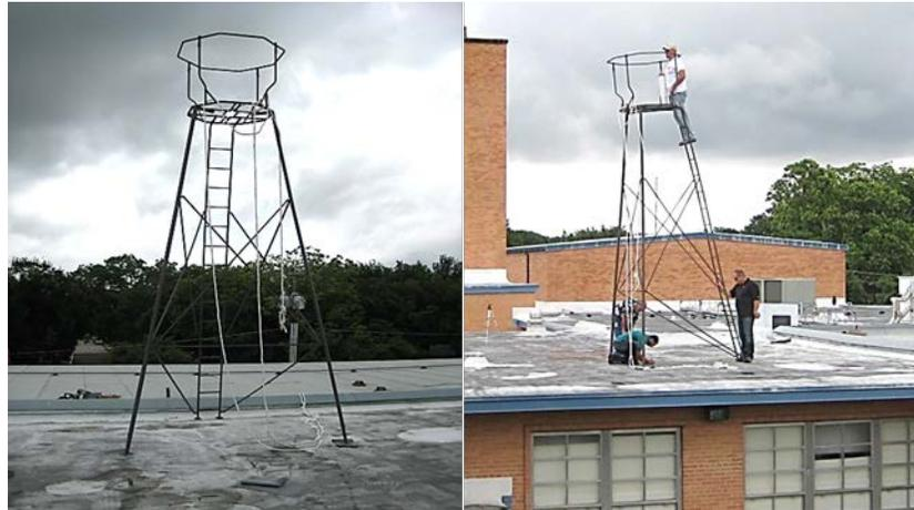
*Figure 1: Hail Testing Apparatus.*
